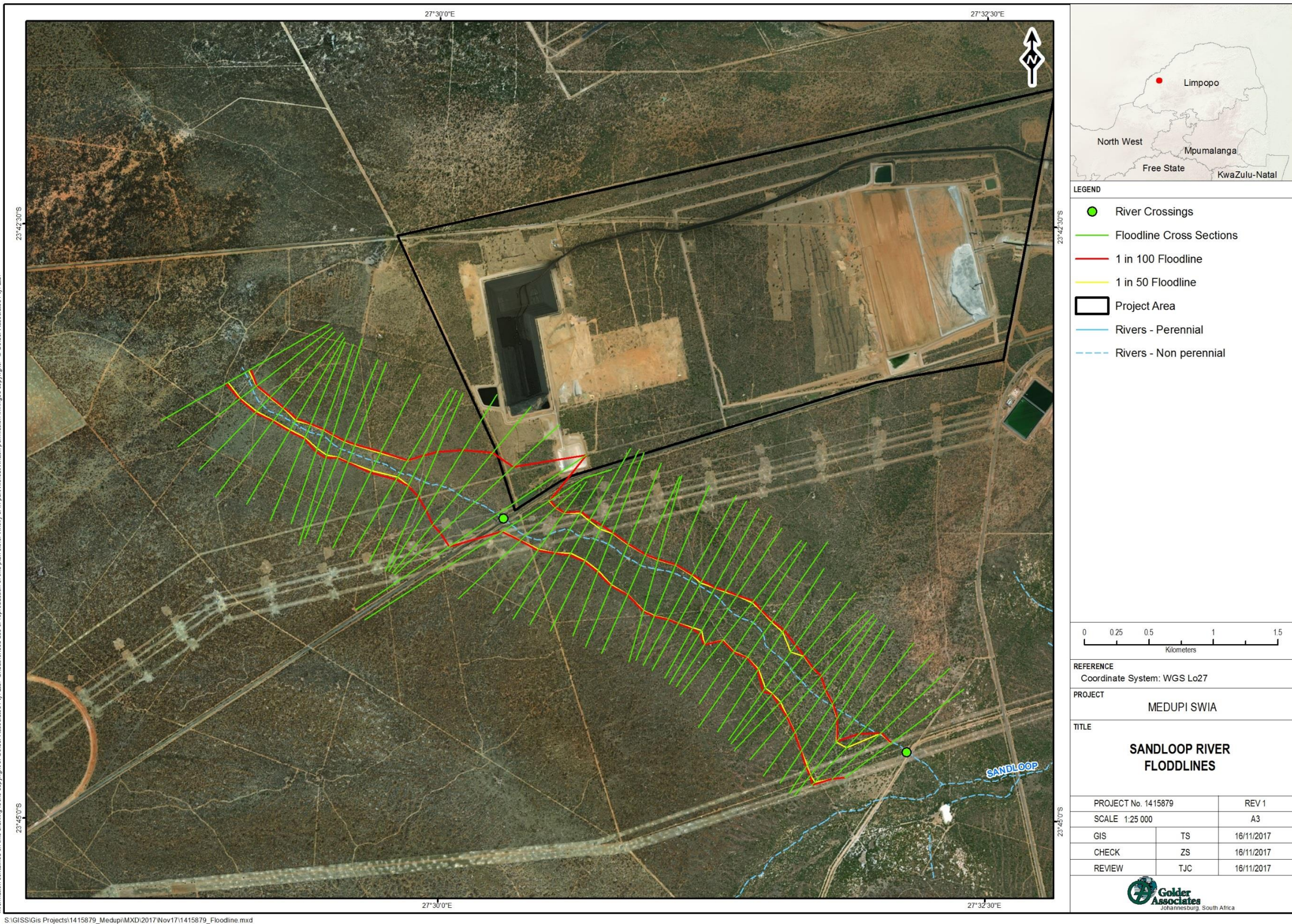
Figure 20: The 1 in 100 year recurrence interval floodline for Sandloop River showing encroachment of the PCD into the floodline
